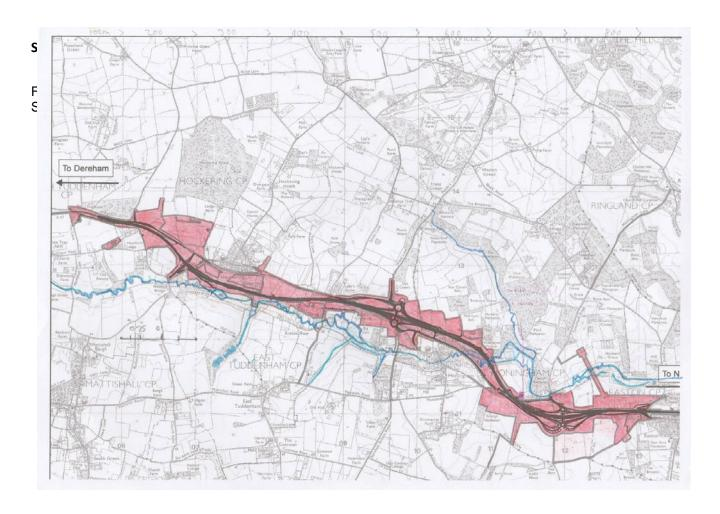
Fig 3. Proposed route of A47NT-E running parallel to the River Tud. Red area is the construction zone and Blue meandering line represents the river. Note the river runs through or next to the construction zone in 5 places and it is also crossed by a major bridge, along this 9km section of road.
